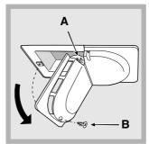
Access the light bulb (A) by unscrewing the fixing screw (B) which is located at the back of the lampcover, as shown (see diagram). Replace it with a similar light bulb, the power of which should not exceed 15W.
